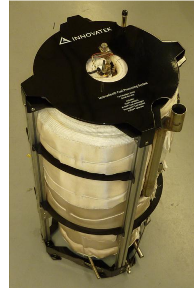
15 kW bio-SPK fuel processor For HT-PEM fuel cell airplane APU, 2012
