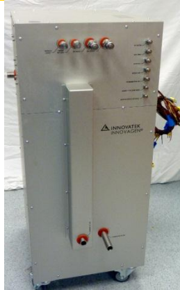
5 kW ULSD fuel processor for HT-PEM fuel cell distributed power generation, 2009
