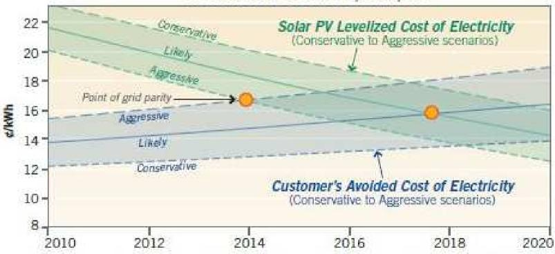
PV cost/performance typical for the Northeast US; Bebt 8% equity 10% (80:20), 10 yrs debt, 25 yr lifetime, 30% ITC (assumed beyond 2016); includes state incentives; 2010 electricity costs are typical for Northeast states with EIA electricity escalation rates.
