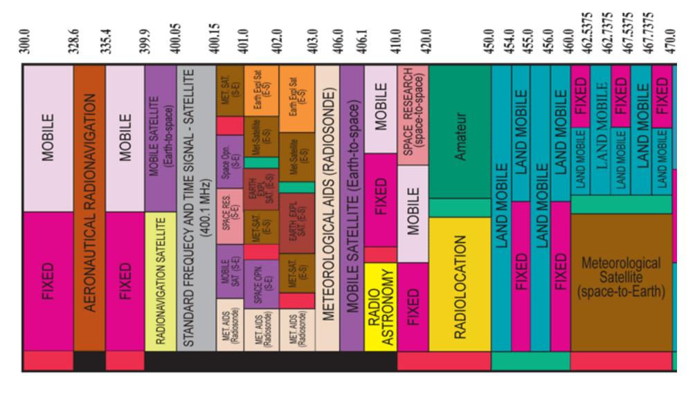
Details of a thin slice, from 300 MHz to 470 MHz
