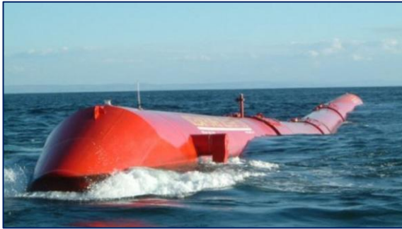
Surface attenuator: Pelamis Wave Power
