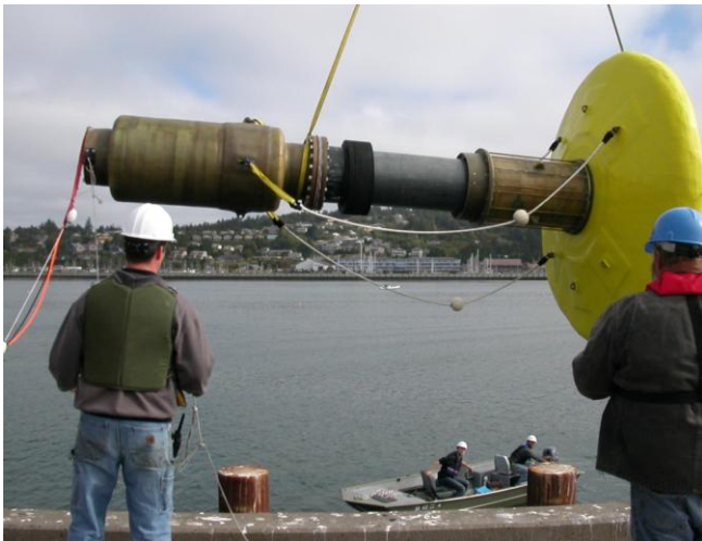
Deployment of 10 kW point absorber off the coast of Newport, OR
