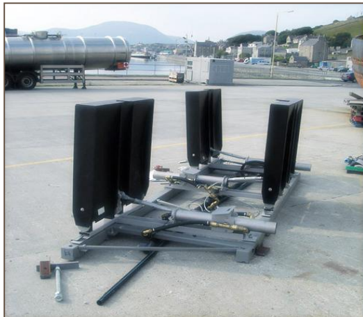
Submerged surge converter: AW Energy
