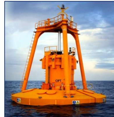
Point absorber: Ocean Power Technologies
