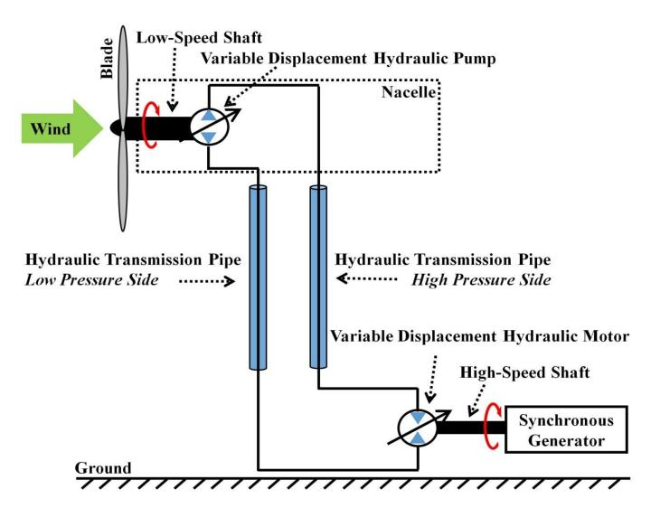
P<sub>wind</sub>: Raw power from wind P<sub>rotor</sub>: Power available at rotor  $\tau_{\text{rotor}}\text{:}$  Torque asserted at rotor C<sub>n</sub>: Power coefficient U: Wind speed A: Swept area R: Blade radius  $\rho_{\text{air}}$ :Air density λ: Tip-speed ratio  $\omega_r$ :Rotor speed J<sub>r</sub>: Rotor inertia V<sub>D</sub>: Pump displacement  $\Delta P_p$ : Differential pressure at pump  $\eta_{\text{mech,p}}$ : Pump mechanical efficiency β:pitch angle
