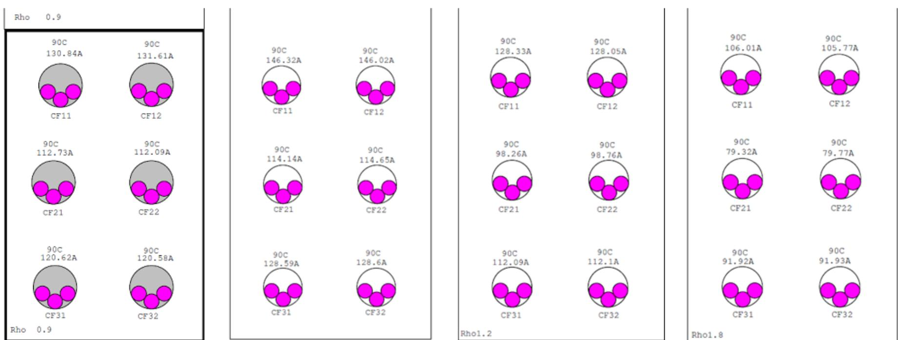
Figure 8. Collector feeders ampacity for cable buried in conduits and direct buried in soil with different Rho.
