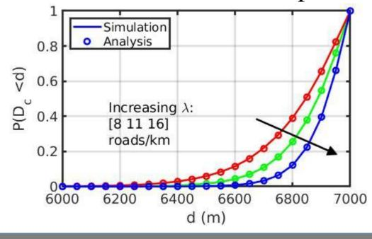
The distribution of the charging distance, i.e.,  $D_c$ , on a 7km trip across the center of cities with different road densities, i.e.,  $\lambda$ , when the source (non-charging) and destination (charging) roads are parallel
