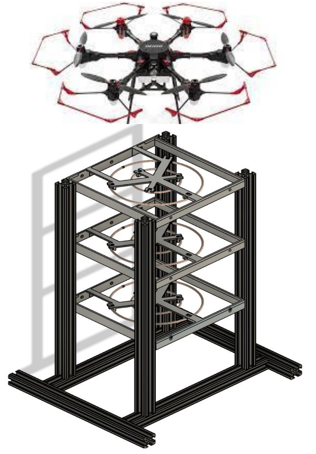
Figure 1: A high-level concept of our CSCMR WPT System
