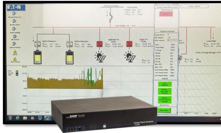
Economic optimization software paired with intelligent microgrid controls manage DERs and utility power
